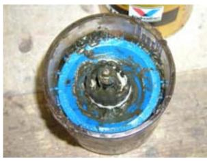
Pack both inner and outer bearings using a high melting point wheel bearing grease. Now is not the time to skimp. Buy the best grease you can find. I have a fancy bearing packer that I like a lot but you can do this without it. Just put a spoon full of grease into the palm of one hand and press the bearing repeatedly into it until you are pushing grease out the top of the bearing.
