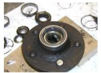
Tighten the spindle nut, and how do you do that? With everything back in place, rotate the wheel and tighten the spindle nut to 12 ft. lbs. of torque. Back off the adjusting nut one flat and insert the cotter pin. Spin the wheel to check that it rolls freely. Bearings should have zero preload and .001 to .008 end movement. Good luck.
