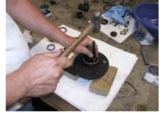
Ok, Now it is time to put it back together. To install the new races in the hub, what I like to do is take the old races and grind down the outer surface so that they are no longer a press fit. Now you can use them as a drift to tap the new races in with out the "drift" getting stuck in the hub.
