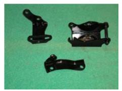
On the left are the correct P/S brackets for 1969. On the right are the correct P/S brackets for 1970.
