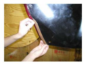
The panel was then clamped into place leaving a small gap for welding
