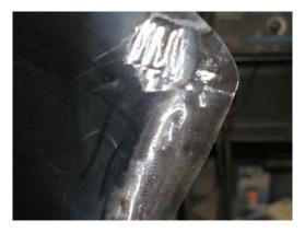
Fill the dimples with weld, being careful to keep moving so as not to burn through
