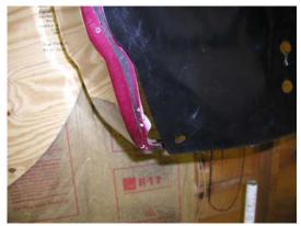
wrong shape. Here we have a picture of a 1970 right front fender with an after market steel inner fender well that meets that criteria. The inner fender well did not match up with the fender. There was a gap between the fender and the inner fender well. What to do??
